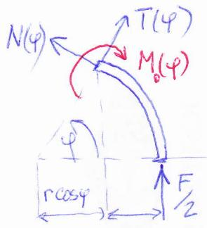
$$M_o(\varphi) = \frac{F}{2}r(1 - \cos\varphi) \quad \frac{\partial M_o(\varphi)}{\partial F} = \frac{1}{2}r(1 - \cos\varphi)$$
