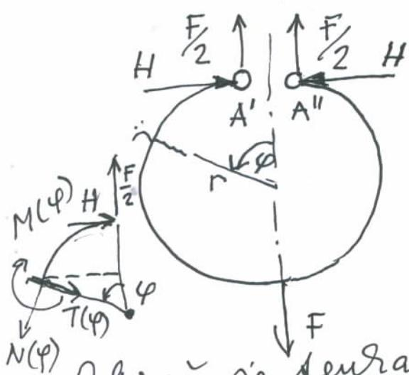
$$\frac{\partial U}{\partial H} = 0 \quad U = \int_{(0)}^{\pi} \frac{M(\varphi)^2}{2EJ} \cdot r d\varphi$$
