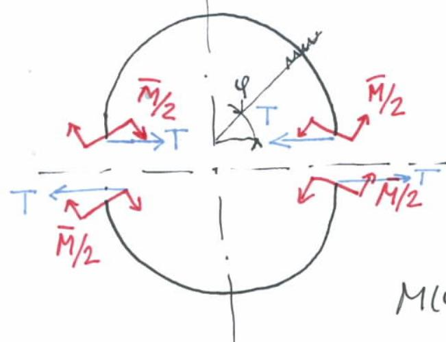
$$M(\varphi) = \frac{\bar{M}}{2} - T \cdot r \sin \varphi, \quad \frac{\partial M(\varphi)}{\partial T} = -r \sin \varphi$$
