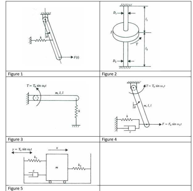
6) In problem 5, determine the steady state amplitude of the force transmitted to the moving base.
