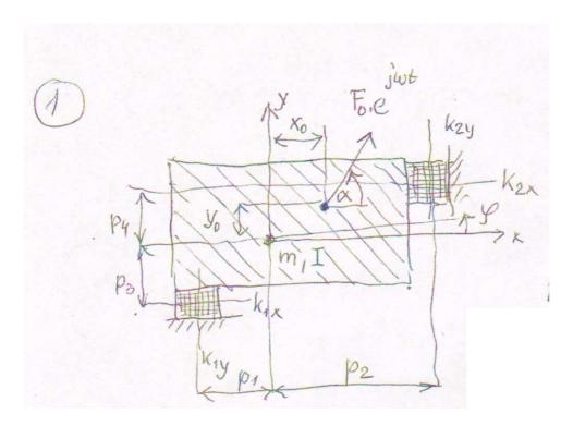
Given: mass m, mass moment of inertia I, stiffnesses  $k_{ix}$ ,  $k_{iy}$ , dimensions  $p_i$  and  $x_0$ ,  $y_0$ ,  $F_0$ , ,  $\alpha$ ,  $\omega$ , constant  $\kappa$  for damping  $B=\kappa.K$
