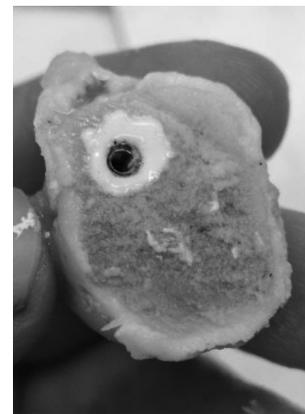
**Figure 2** - Test specimen (implant fixed in bone with cement)
