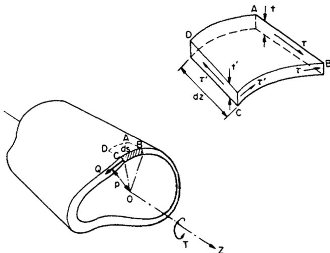
Fig. 5.6. Thin-walled closed section subjected to axial torque.
